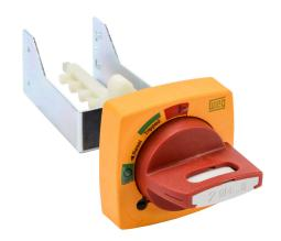
WEG Electric rotary handle, selector, red/yellow, external front mount, 2-position, lockable in OFF only, defeatable, NEMA 4/4X, IP65. For use with MPW40 series manual motor protectors. 130mm shaft included.
