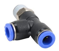
NITRA pneumatic push-to-connect fitting, run tee, rotating, thermoplastic (PBT) body, nickel-plated brass threads, thread sealant, (1) R1/4 male BSPT to (2) 5/16in (8mm) push-to-connect. Package of 5.
