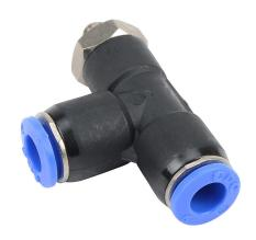
NITRA pneumatic push-to-connect fitting, run tee, rotating, thermoplastic (PBT) body, nickel-plated brass threads, thread sealant, (1) M5 x 0.8 male ISO to (2) 6mm push-to-connect. Package of 5.
