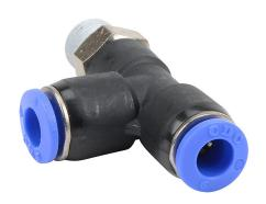
NITRA pneumatic push-to-connect fitting, run tee, rotating, thermoplastic (PBT) body, nickel-plated brass threads, thread sealant, (1) R1/8 male BSPT to (2) 6mm push-to-connect. Package of 5.
