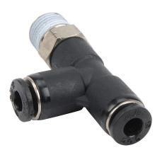
NITRA pneumatic push-to-connect fitting, male, run tee, rotating, thermoplastic (PBT) body, nickel-plated brass threads, (2) 5/32in (4mm) tube to 1/8in NPT connection(s). Package of 5.
