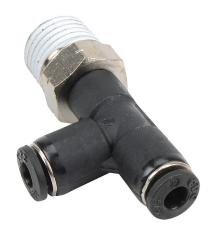
NITRA pneumatic push-to-connect fitting, run tee, rotating, thermoplastic (PBT) body, nickel-plated brass threads, thread sealant, (1) 1/4in male NPT to (2) 5/32in (4mm) push-to-connect. Package of 5.
