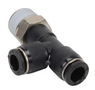
NITRA pneumatic push-to-connect fitting, run tee, rotating, thermoplastic (PBT) body, nickel-plated brass threads, thread sealant, (1) 3/8in male NPT to (2) 5/16in (8mm) push-to-connect. Package of 5.
