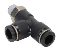
NITRA pneumatic push-to-connect fitting, run tee, rotating, thermoplastic (PBT) body, nickel-plated brass threads, thread sealant, (1) 1/8in male NPT to (2) 5/16in (8mm) push-to-connect. Package of 5.
