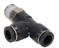
NITRA pneumatic push-to-connect fitting, run tee, rotating, thermoplastic (PBT) body, nickel-plated brass threads, thread sealant, (1) 1/4in male NPT to (2) 5/16in (8mm) push-to-connect. Package of 5.
