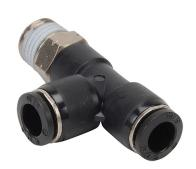
NITRA pneumatic push-to-connect fitting, male, run tee, rotating, thermoplastic (PBT) body, nickel-plated brass threads, (2) 5/16in (8mm) tube to 1/4in NPT connection(s). Package of 5.
