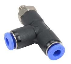
NITRA pneumatic push-to-connect fitting, run tee, rotating, thermoplastic (PBT) body, nickel-plated brass threads, thread sealant, (1) M5 x 0.8 male ISO to (2) 5/32in (4mm) push-to-connect. Package of 5.
