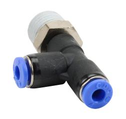
NITRA pneumatic push-to-connect fitting, run tee, rotating, thermoplastic (PBT) body, nickel-plated brass threads, thread sealant, (1) R1/4 male BSPT to (2) 5/32in (4mm) push-to-connect. Package of 5.
