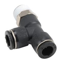
NITRA pneumatic push-to-connect fitting, run tee, rotating, thermoplastic (PBT) body, nickel-plated brass threads, thread sealant, (2) 3/8in push-to-connect to (1) 3/8in male NPT. Package of 5.
