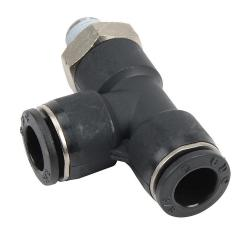
NITRA pneumatic push-to-connect fitting, run tee, rotating, thermoplastic (PBT) body, nickel-plated brass threads, thread sealant, (2) 3/8in push-to-connect to (1) 1/8in male NPT. Package of 5.
