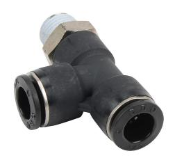
NITRA pneumatic push-to-connect fitting, run tee, rotating, thermoplastic (PBT) body, nickel-plated brass threads, thread sealant, (1) 1/4in male NPT to (2) 3/8in push-to-connect. Package of 5.
