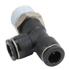
NITRA pneumatic push-to-connect fitting, run tee, rotating, thermoplastic (PBT) body, nickel-plated brass threads, thread sealant, (1) 1/2in male NPT to (2) 3/8in push-to-connect. Package of 5.
