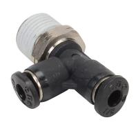
NITRA pneumatic push-to-connect fitting, run tee, rotating, thermoplastic (PBT) body, nickel-plated brass threads, thread sealant, (1) 1/8in male NPT to (2) 1/8in push-to-connect. Package of 5.
