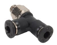
NITRA pneumatic push-to-connect fitting, run tee, rotating, thermoplastic (PBT) body, nickel-plated brass threads, thread sealant, (1) #10-32 male UNF to (2) 1/8in push-to-connect. Package of 5.
