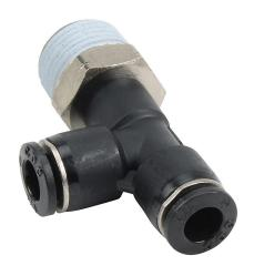
NITRA pneumatic push-to-connect fitting, run tee, rotating, thermoplastic (PBT) body, nickel-plated brass threads, thread sealant, (1) 3/8in male NPT to (2) 1/4in push-to-connect. Package of 5.
