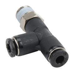
NITRA pneumatic push-to-connect fitting, run tee, rotating, thermoplastic (PBT) body, nickel-plated brass threads, thread sealant, (1) 1/8in male NPT to (2) 1/4in push-to-connect. Package of 5.
