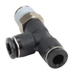
NITRA pneumatic push-to-connect fitting, run tee, rotating, thermoplastic (PBT) body, nickel-plated brass threads, thread sealant, (1) 1/4in male NPT to (2) 1/4in push-to-connect. Package of 5.
