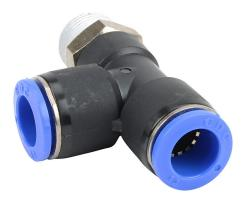
NITRA pneumatic push-to-connect fitting, run tee, rotating, thermoplastic (PBT) body, nickel-plated brass threads, thread sealant, (1) R3/8 male BSPT to (2) 12mm push-to-connect. Package of 5.
