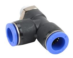
NITRA pneumatic push-to-connect fitting, run tee, rotating, thermoplastic (PBT) body, nickel-plated brass threads, thread sealant, (1) R1/4 male BSPT to (2) 12mm push-to-connect. Package of 5.
