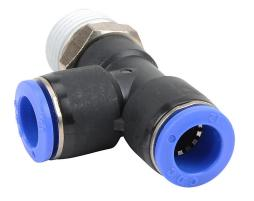
NITRA pneumatic push-to-connect fitting, run tee, rotating, thermoplastic (PBT) body, nickel-plated brass threads, thread sealant, (1) R1/2 male BSPT to (2) 12mm push-to-connect. Package of 5.
