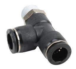
NITRA pneumatic push-to-connect fitting, run tee, rotating, thermoplastic (PBT) body, nickel-plated brass threads, thread sealant, (1) 3/8in male NPT to (2) 1/2in push-to-connect. Package of 5.
