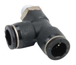
NITRA pneumatic push-to-connect fitting, male, run tee, rotating, thermoplastic (PBT) body, nickel-plated brass threads, (2) 1/2in tube to 1/4in NPT connection(s). Package of 5.
