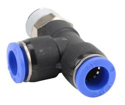
NITRA pneumatic push-to-connect fitting, run tee, rotating, thermoplastic (PBT) body, nickel-plated brass threads, thread sealant, (1) R3/8 male BSPT to (2) 10mm push-to-connect. Package of 5.
