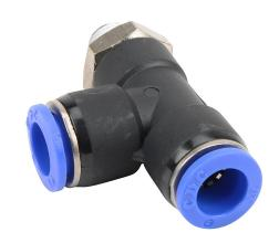
NITRA pneumatic push-to-connect fitting, run tee, rotating, thermoplastic (PBT) body, nickel-plated brass threads, thread sealant, (1) R1/8 male BSPT to (2) 10mm push-to-connect. Package of 5.
