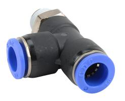
NITRA pneumatic push-to-connect fitting, run tee, rotating, thermoplastic (PBT) body, nickel-plated brass threads, thread sealant, (1) R1/4 male BSPT to (2) 10mm push-to-connect. Package of 5.
