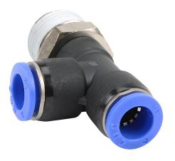
NITRA pneumatic push-to-connect fitting, run tee, rotating, thermoplastic (PBT) body, nickel-plated brass threads, thread sealant, (1) R1/2 male BSPT to (2) 10mm push-to-connect. Package of 5.
