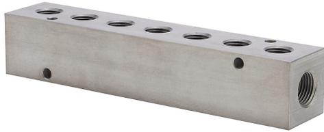
NITRA pneumatic valve manifold, stainless steel, silver, rectangular, 3500 psi maximum operating pressure, (7) stations, (2) 3/8in female NPT inlet(s), (7) 1/4in female NPT outlet(s), standard hole spacing.
