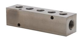
NITRA pneumatic valve manifold, stainless steel, rectangular, 3500 psi maximum operating pressure, (5) stations, (2) 3/8in female NPT inlet(s), (5) 1/4in female NPT outlet(s), standard hole spacing.
