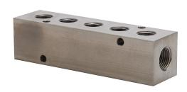
NITRA pneumatic valve manifold, stainless steel, silver, rectangular, 3500 psi maximum operating pressure, (5) stations, (2) 3/8in female NPT inlet(s), (5) 1/4in female NPT outlet(s), standard hole spacing.
