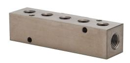
NITRA pneumatic valve manifold, stainless steel, silver, rectangular, 3500 psi maximum operating pressure, (5) stations, (2) 1/4in female NPT inlet(s), (5) 1/8in female NPT outlet(s), standard hole spacing.
