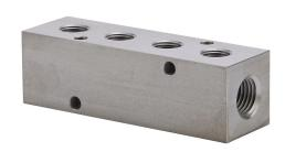
NITRA pneumatic valve manifold, stainless steel, rectangular, 3500 psi maximum operating pressure, (4) stations, (2) 1/4in female NPT inlet(s), (4) 1/8in female NPT outlet(s), standard hole spacing.
