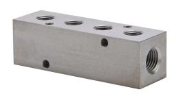
NITRA pneumatic valve manifold, stainless steel, silver, rectangular, 3500 psi maximum operating pressure, (4) stations, (2) 1/4in female NPT inlet(s), (4) 1/8in female NPT outlet(s), standard hole spacing.
