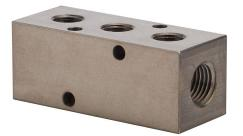
NITRA pneumatic valve manifold, stainless steel, silver, rectangular, 3500 psi maximum operating pressure, (3) stations, (2) 1/4in female NPT inlet(s), (3) 1/8in female NPT outlet(s), standard hole spacing.
