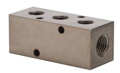
NITRA pneumatic valve manifold, stainless steel, rectangular, 3500 psi maximum operating pressure, (3) stations, (2) 1/4in female NPT inlet(s), (3) 1/8in female NPT outlet(s), standard hole spacing.
