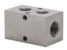
NITRA pneumatic valve manifold, stainless steel, silver, rectangular, 3500 psi maximum operating pressure, (2) stations, (2) 3/8in female NPT inlet(s), (2) 1/4in female NPT outlet(s), standard hole spacing.
