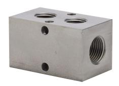
NITRA pneumatic valve manifold, stainless steel, rectangular, 3500 psi maximum operating pressure, (2) stations, (2) 3/8in female NPT inlet(s), (2) 1/4in female NPT outlet(s), standard hole spacing.
