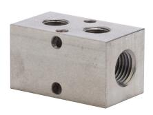
NITRA pneumatic valve manifold, stainless steel, silver, rectangular, 3500 psi maximum operating pressure, (2) stations, (2) 1/4in female NPT inlet(s), (2) 1/8in female NPT outlet(s), standard hole spacing.
