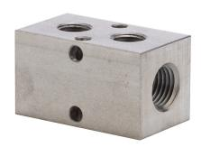
NITRA pneumatic valve manifold, stainless steel, rectangular, 3500 psi maximum operating pressure, (2) stations, (2) 1/4in female NPT inlet(s), (2) 1/8in female NPT outlet(s), standard hole spacing.
