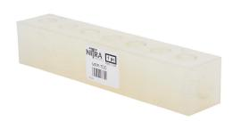
NITRA pneumatic or water valve manifold, polypropylene (PP), white, rectangular, 150 psi maximum operating pressure, (7) stations, (2) 3/8in female NPT inlet(s), (7) 1/4in female NPT outlet(s), standard hole spacing.
