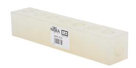
NITRA pneumatic or water valve manifold, polypropylene (PP), rectangular, 150 psi maximum operating pressure, (7) stations, (2) 3/8in female NPT inlet(s), (7) 1/4in female NPT outlet(s), standard hole spacing.
