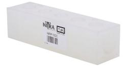
NITRA pneumatic or water valve manifold, polypropylene (PP), white, rectangular, 150 psi maximum operating pressure, (5) stations, (2) 3/8in female NPT inlet(s), (5) 1/4in female NPT outlet(s), standard hole spacing.
