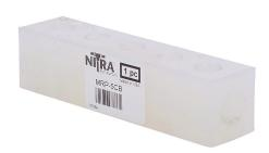
NITRA pneumatic or water valve manifold, polypropylene (PP), rectangular, 150 psi maximum operating pressure, (5) stations, (2) 1/4in female NPT inlet(s), (5) 1/8in female NPT outlet(s), standard hole spacing.
