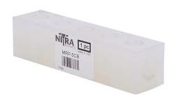
NITRA pneumatic or water valve manifold, polypropylene (PP), white, rectangular, 150 psi maximum operating pressure, (5) stations, (2) 1/4in female NPT inlet(s), (5) 1/8in female NPT outlet(s), standard hole spacing.
