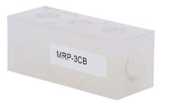
NITRA pneumatic or water valve manifold, polypropylene (PP), white, rectangular, 150 psi maximum operating pressure, (3) stations, (2) 1/4in female NPT inlet(s), (3) 1/8in female NPT outlet(s), standard hole spacing.
