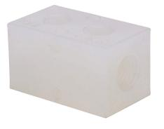
NITRA pneumatic or water valve manifold, polypropylene (PP), rectangular, 150 psi maximum operating pressure, (2) stations, (2) 1/4in female NPT inlet(s), (2) 1/8in female NPT outlet(s), standard hole spacing.
