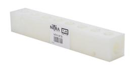
NITRA pneumatic or water valve manifold, Nylon 6, white, rectangular, 200 psi maximum operating pressure, (8) stations, (2) 1/4in female NPT inlet(s), (8) 1/8in female NPT outlet(s), standard hole spacing.
