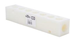
NITRA pneumatic or water valve manifold, Nylon 6, white, rectangular, 200 psi maximum operating pressure, (7) stations, (2) 3/8in female NPT inlet(s), (7) 1/4in female NPT outlet(s), standard hole spacing.
