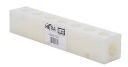
NITRA pneumatic or water valve manifold, Nylon 6, white, rectangular, 200 psi maximum operating pressure, (7) stations, (2) 1/4in female NPT inlet(s), (7) 1/8in female NPT outlet(s), standard hole spacing.
