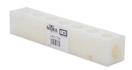
NITRA pneumatic or water valve manifold, Nylon 6, rectangular, 200 psi maximum operating pressure, (7) stations, (2) 1/4in female NPT inlet(s), (7) 1/8in female NPT outlet(s), standard hole spacing.
