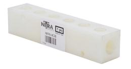
NITRA pneumatic or water valve manifold, Nylon 6, white, rectangular, 200 psi maximum operating pressure, (6) stations, (2) 1/4in female NPT inlet(s), (6) 1/8in female NPT outlet(s), standard hole spacing.
