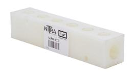
NITRA pneumatic or water valve manifold, Nylon 6, rectangular, 200 psi maximum operating pressure, (6) stations, (2) 1/4in female NPT inlet(s), (6) 1/8in female NPT outlet(s), standard hole spacing.
