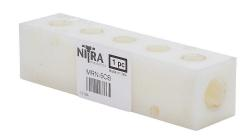
NITRA pneumatic or water valve manifold, Nylon 6, white, rectangular, 200 psi maximum operating pressure, (5) stations, (2) 1/4in female NPT inlet(s), (5) 1/8in female NPT outlet(s), standard hole spacing.
