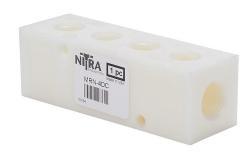
NITRA pneumatic or water valve manifold, Nylon 6, rectangular, 200 psi maximum operating pressure, (4) stations, (2) 3/8in female NPT inlet(s), (4) 1/4in female NPT outlet(s), standard hole spacing.
