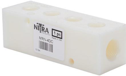
NITRA pneumatic or water valve manifold, Nylon 6, white, rectangular, 200 psi maximum operating pressure, (4) stations, (2) 3/8in female NPT inlet(s), (4) 1/4in female NPT outlet(s), standard hole spacing.
