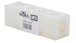
NITRA pneumatic or water valve manifold, Nylon 6, white, rectangular, 200 psi maximum operating pressure, (4) stations, (2) 1/4in female NPT inlet(s), (4) 1/8in female NPT outlet(s), standard hole spacing.
