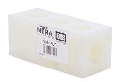
NITRA pneumatic or water valve manifold, Nylon 6, white, rectangular, 200 psi maximum operating pressure, (3) stations, (2) 3/8in female NPT inlet(s), (3) 1/4in female NPT outlet(s), standard hole spacing.
