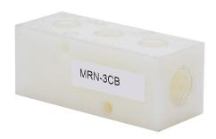
NITRA pneumatic or water valve manifold, Nylon 6, rectangular, 200 psi maximum operating pressure, (3) stations, (2) 1/4in female NPT inlet(s), (3) 1/8in female NPT outlet(s), standard hole spacing.
